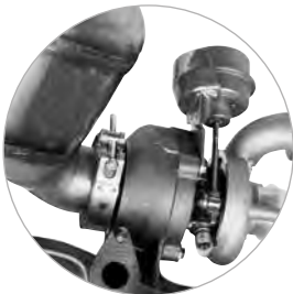
Automotive: Turbocharger – catalytic converter connection
